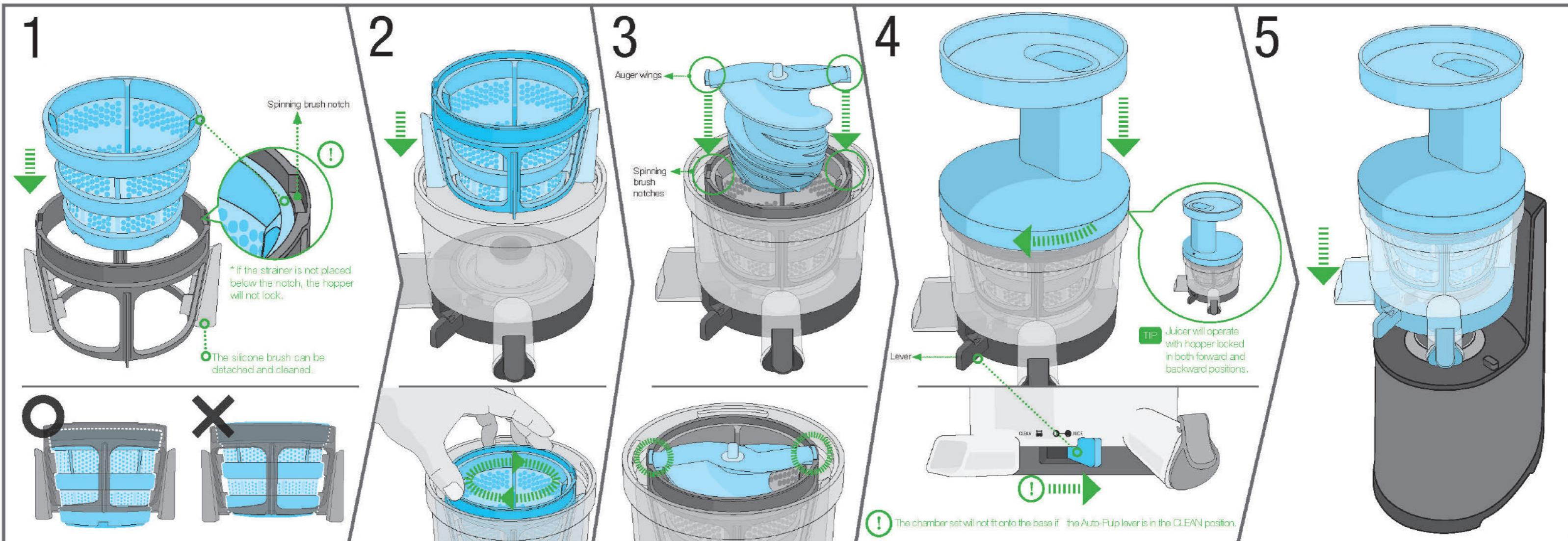
Place strainer into spinning brush. Press strainer down inside spinning brush until the upper edge of the strainer is below the notches in the top of the spinning brush.
