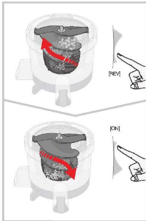
**1** Press [REV] for 3-4 seconds to release pressure from chamber set. Repeat if necessary.
