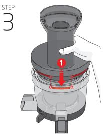
Assemble the hopper as shown. Place the hopper on the chamber and turn clockwise until it is completely locked.
