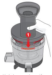
Assemble the hopper as shown. After fitting the hopper on the chamber, turn clockwise until it locks completely.
