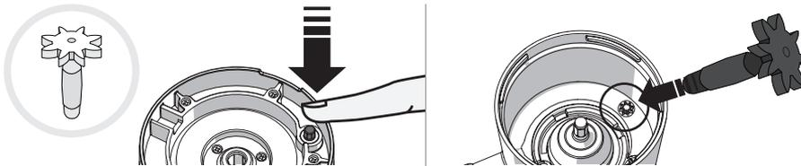
Push the intermediate gear from the bottom side of the chamber to remove the gear.
