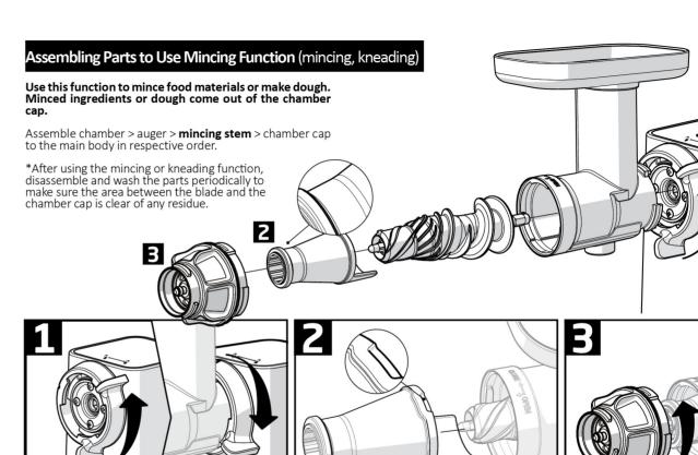
Turn the locking Clip of the main body counterclockwise ( → )to open, place the chamber, and turn the locking Clip ( → )clockwise to lock.  Assemble auger > mincing stem to the chamber assembly in respective order. Place the auger until its shaft completely fits into the main body. Make sure the groove on the mincing stem faces up when assembling the parts.
