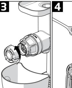
Select a nozzle that is suitable for the shape of a noodle you want to make and connect it to the chamber cap.
