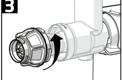
3. Turn the chamber cap counterclockwise (**CLOSE**) to fit.
