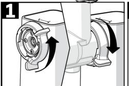
Turn the locking Clip of the main body counterclockwise ( → )to open, place the chamber, and turn the locking Clip ( → )clockwise to lock.
