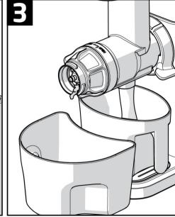
Dregs are discharged through the chamber cap and the juice is extracted through the juice outlet on the bottom of the chamber.
