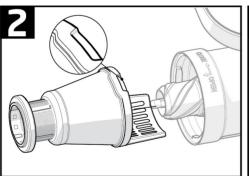
2. Assemble auger > juicing stem to the chamber assembly in respective order. Place the auger until its shaft completely fits into the main body. Make sure the groove on the juicing stem faces up when assembling the parts.
