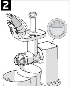
Insert ingredients into the inlet and press [ON] button on the back of the main body. Press the ingredients down with the pusher to ease the insertion.
