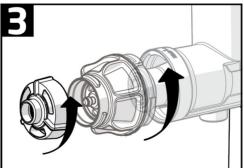
3. Turn the chamber cap counterclockwise (CLOSE) to fit. Select a nozzle that is suitable for the shape of a noodle you want to make and connect it to the chamber cap.
